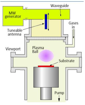
**Figure 7.** Microwave (MW) plasma CVD reactor. MW radiation enters the chamber via a waveguide and an antenna. The chamber forms a resonant cavity that is tuned by moving the antenna position. The MW power generates a plasma situated just above the substrate surface which activates, ionises and dissociates the input gases, initiating diamond growth on the nearby substrate. Reproduced with permission from ref 39. Copyright 1999 University of Bristol.
