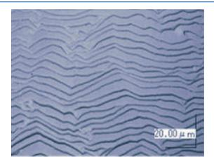
Figure 11. SEM image illustrating the characteristic macroscopic stepbunching seen on the surface of SCD samples grown using nitrogencontaining gas mixtures. Reprinted with permission from ref 88. Copyright 2016 Japan Society of Applied Physics.
