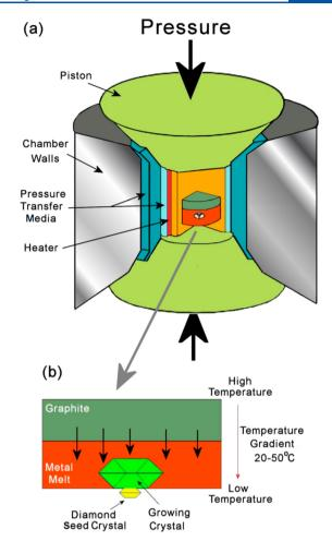
Figure 5. Schematic diagram of (a) an HPHT press, wherein a cell containing graphite, a metal melt, and a diamond seed crystal is subjected to high pressures and temperatures. Under these conditions, (b) the graphite dissolves in the metal and precipitates on the seed crystal, propagating the diamond lattice.
